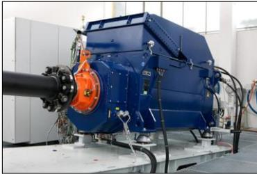
Fig.3: 2 MW/10 kV WT DSgen-set<sup>®</sup> prototype on the test bed.
