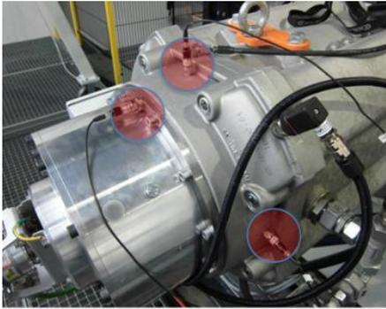
Fig. 9: Measurement points for validation tests
