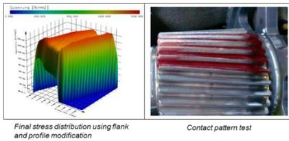
Fig. 11: Micropitting reduction method
