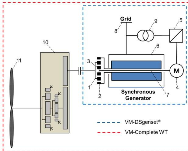
Fig.1: Principal Design of DSGen-set® based on WT and VM
