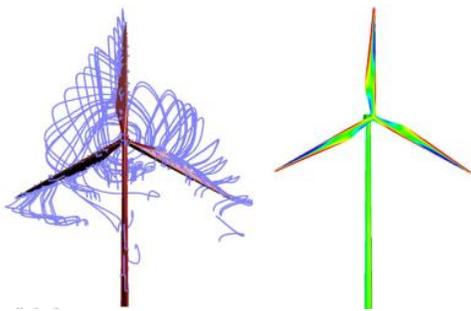
Fig. 13: CFD generated loads on WT blades
