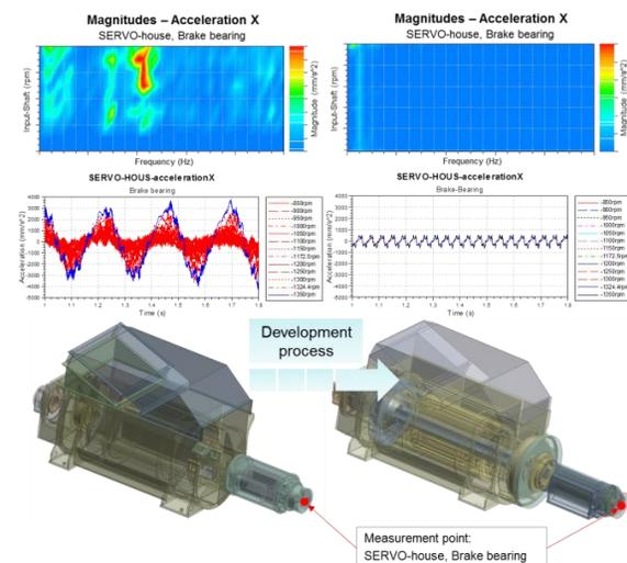
Fig. 8: Elimination of dangerous resonances in VM
