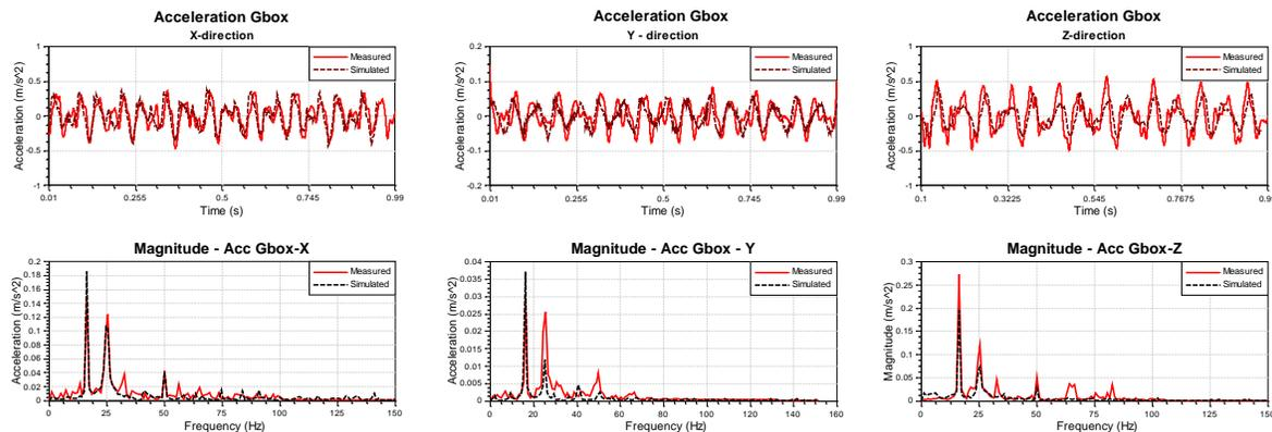
Fig. 10: Comparison of a measurement point in validation tests
