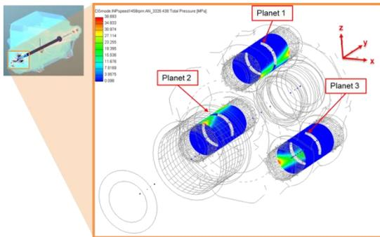
Fig. 12: Plain bearing as an alternative in planetary set
