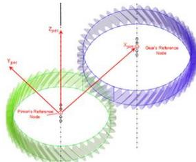
Fig. 6 AVL EXCITE sliced contact gear mesh model
