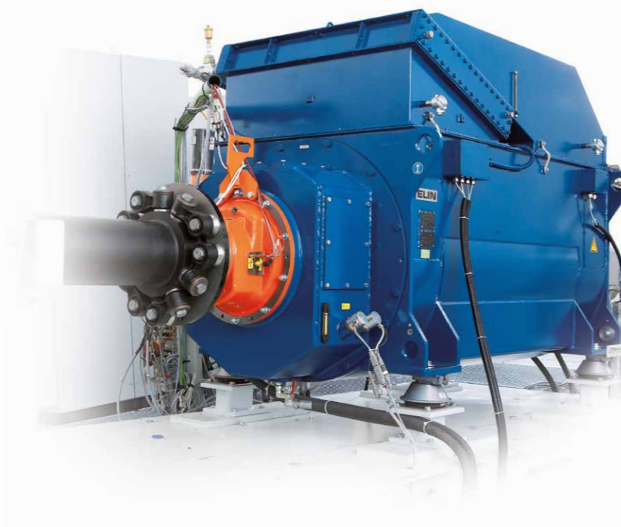
2MW DSgen-set® prototype on the SET test bench in Klagenfurt
